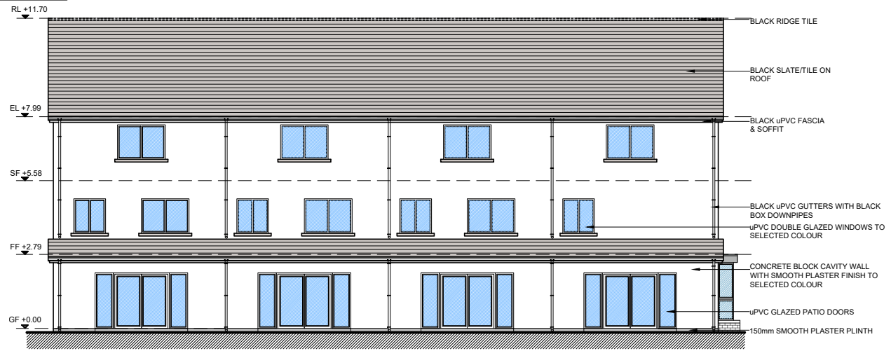
Rear Elevation - Terrace 01 SCALE 1:200 @ A3
